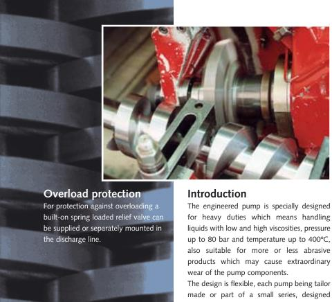
for heavy duties which means handling liquids with low and high viscosities, pressure up to 80 bar and temperature up to 400°C, also suitable for more or less abrasive products which may cause extraordinary
